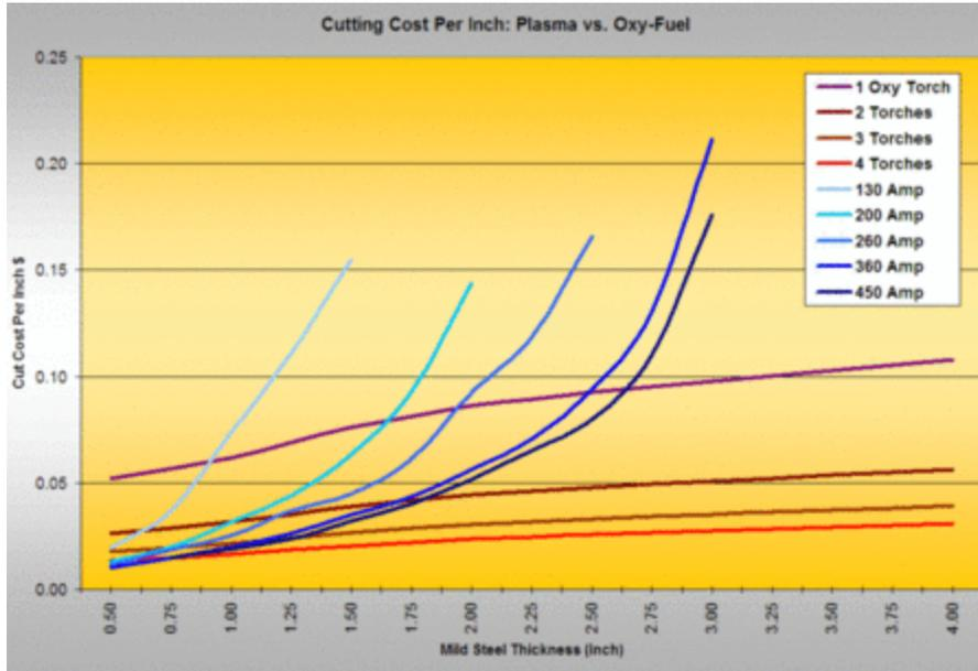
In the next chart, I added calculations that take into account almost all of the costs associated with each process. For plasma, this included electrodes, nozzles, shields, retainers, baffles, and torch coolant, as well as electricity, oxygen, and compressed air. For oxy-fuel, this includes internal and external
