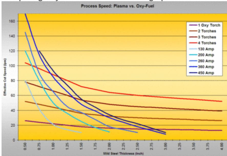
I wanted to take a data driven look at the two processes, to see if there was an obvious cross-over point where one process makes more economical sense than the other. To do that, I charted industry standard cutting speeds for the range of mild steel plate thickness between 1/2 inch and 4 inch, since that would be more than enough to cover the entire range that can be handled by both processes.
