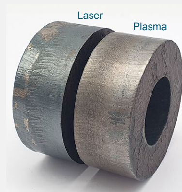
Comparison of cut surfaces 1 inch mild steel
